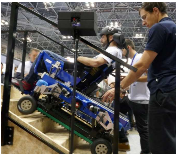
Demonstration of the wheelchair going up the stairs
